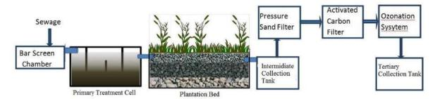
This technology will also be deployed at selected stations and depot for on-site treatment and disposal of human generated waste. Root Zone Treatment of sewage has below advantages over conventional sewage treatment:
